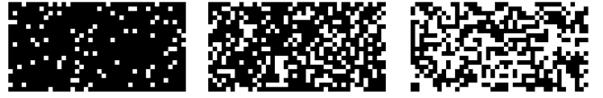
Fig. 1. Examples of the Multi-CCS (M-CCS) implementation that are randomly created with 0.1, 0.3, and 0.5 filling rates ( \nu ), from left to right. These CCSs have dimensions 20 mm \times 10 mm with 40 \times 20 pixels.
